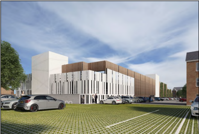
Cladding system and timber screen as viewed from Cotton Lane and from within the site
